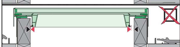
**US** Place the FXC skylight over the curb. Watch and make sure the gaps between the inside of the curb and the skylight's frame are equal.
