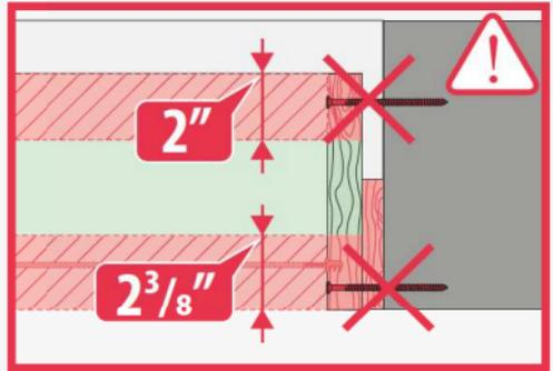
US The stairs must not be used unless they are anchored to the ceiling in accordance with the instructions shown above.
