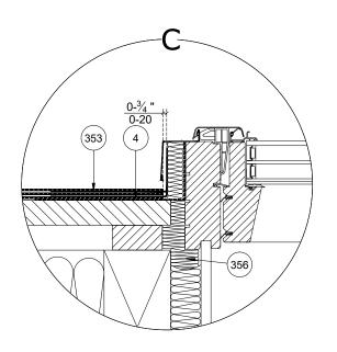
4- ice and water guard by others 28-FTT U6 pivot window FAKRO 38-Installation bracket 353-ELV-AT THERMO flashing side element FAKRO 354-ELV-AT THERMO flashing lower element FAKRO
