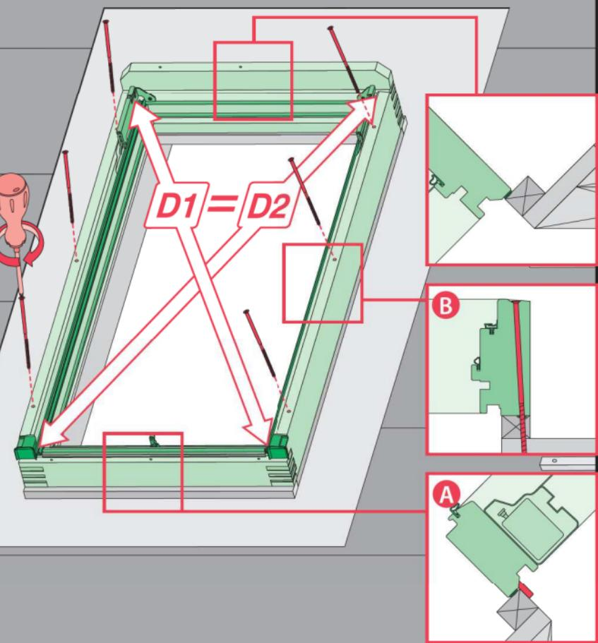
**US** Place the skylight over the rough opening and secure on both sides with screws provided through the pre-drilled holes in the frame. Make sure the diagonals are equal.
