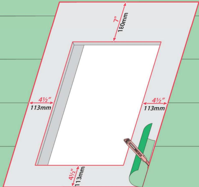
**US** Remove existing roofing underlayment around the opening.
