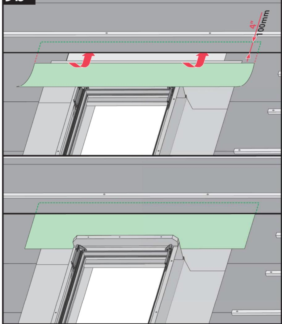
US To ensure proper water drainage, interweave the skylight's underlayment with the new roof underlayment (new construction).
