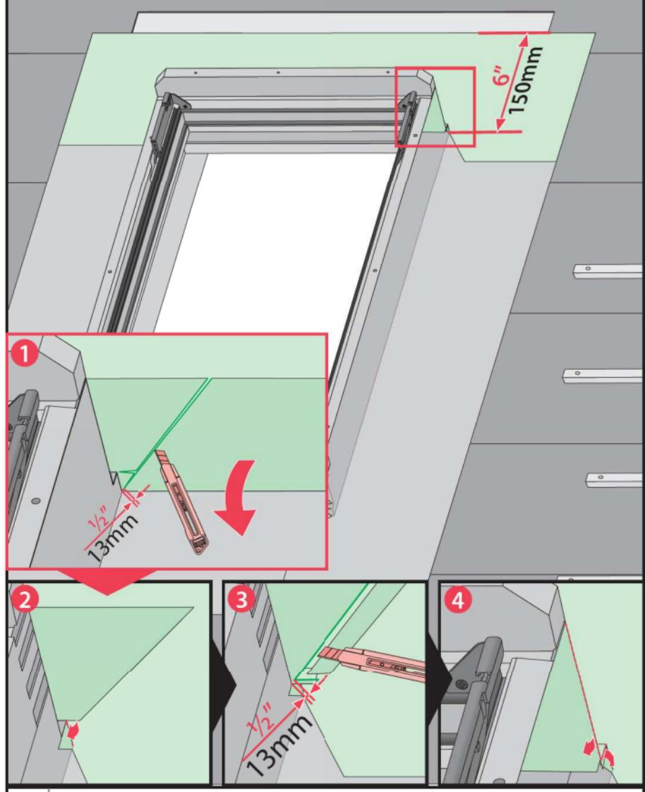
US Wrap the top and corners of the frame overlapping the underlayment.
