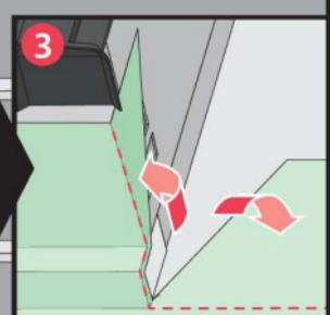
**US** For complete waterproofing, apply self-adhesive roofing underlayment also called Ice & Water Guard. Wrap the bottom frame with corners first. Keep minimum 4" (100mm)overlap with existing roofing underlayment.
