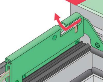
US Lift the sash up high enough to reach hinge lever (1). Lift left and right hinge levers (1) upwards and remove the sash in direction of the arrow (2). Set the sash aside.
