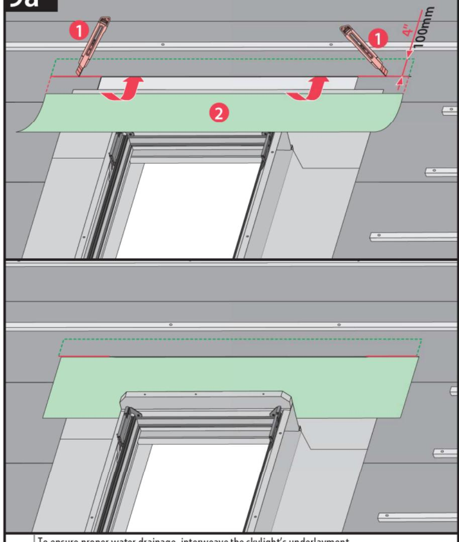
US To ensure proper water drainage, interweave the skylight's underlayment with the existing roof underlayment (retrofit).
