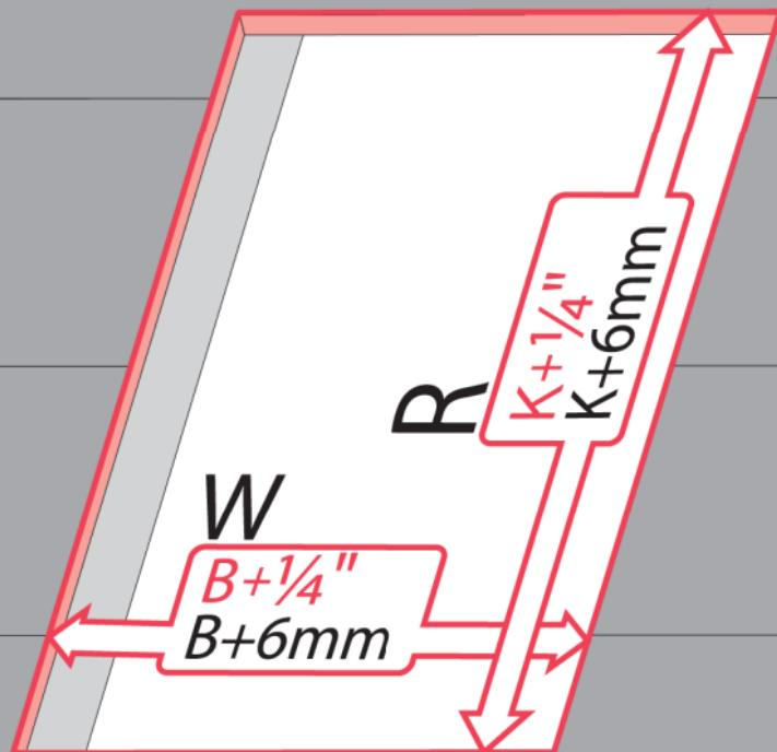
**US** Check the dimensions of the rough opening according to the table at the beginning of the instruction.
