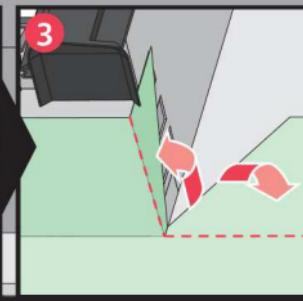
**US** For complete waterproofing, apply self-adhesive roofing underlayment also called Ice & Water Guard. Wrap the bottom frame with corners first. Keep minimum 4" (100mm)overlap with existing roofing underlayment.
