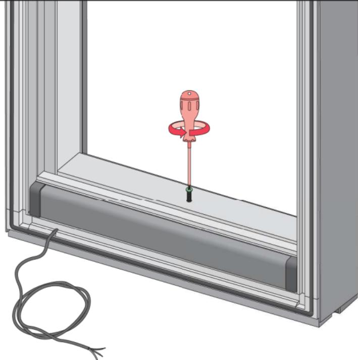
US Unscrew and set aside the screw on the bottom of the sash.
