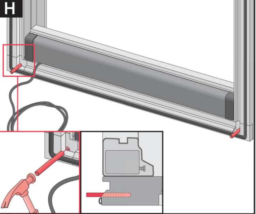
US Insert two metal pins into pre-drilled holes at the bottom of the skylight.
