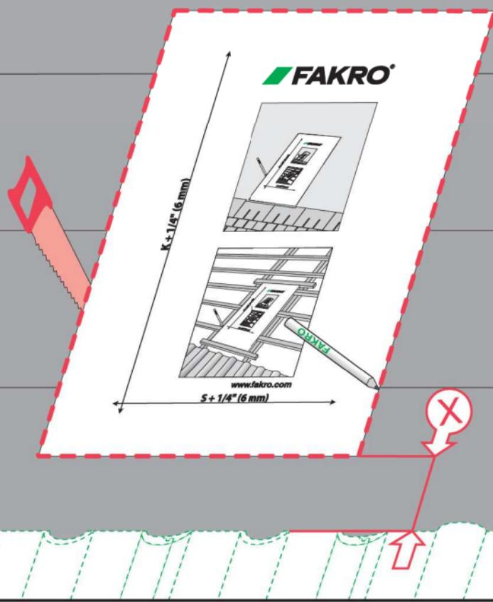
**US** Remove the battens and set aside. Using the template (included) mark the rough opening and cut it out according to the traced lines. Cut very close but inside the traced lines. Keep the required distance from the roofing material.
