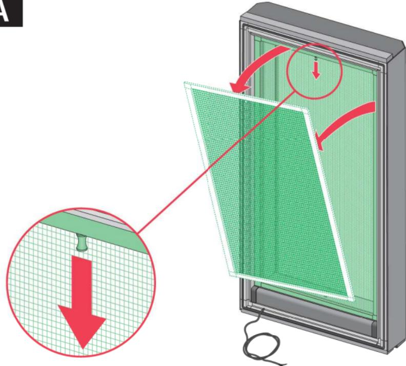
US Pull out bolts and remove the mosquito screen. Set aside.
