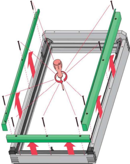
US Remove the side and bottom profiles covering the frame and set them aside.
