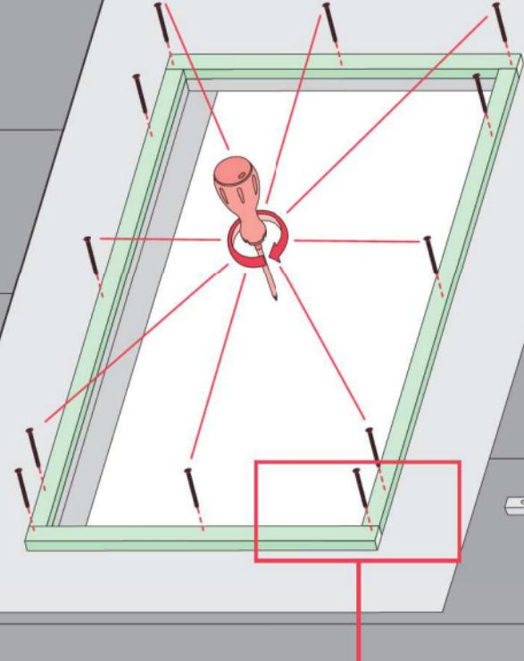
US Place 1 1/4" (30mm) wide battens around the rough opening. Battens should be of the same thickness as battens used for roofing material.
