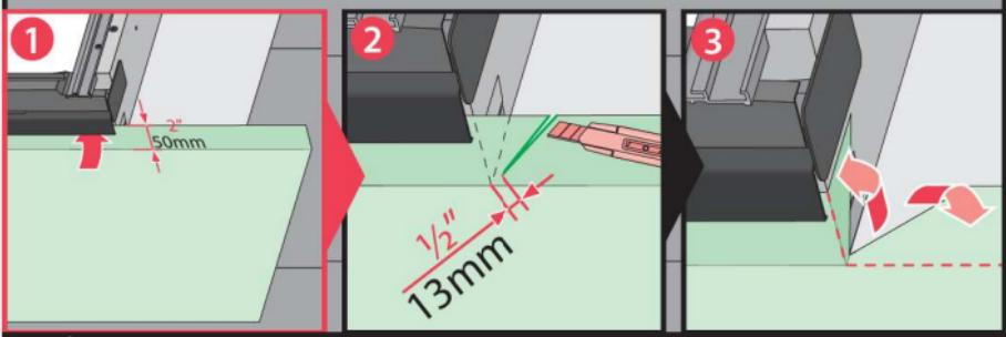
**US** For complete waterproofing, apply self-adhesive roofing underlayment also called Ice & Water Guard. Wrap the bottom frame with corners first. Keep minimum 4" (100mm)overlap with existing roofing underlayment.
