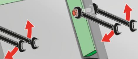
**US** Drill a second hole on each side, and secure with a bolt.
