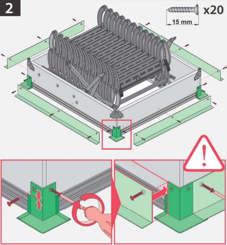
US Tighten the threaded rods securely at each corner
