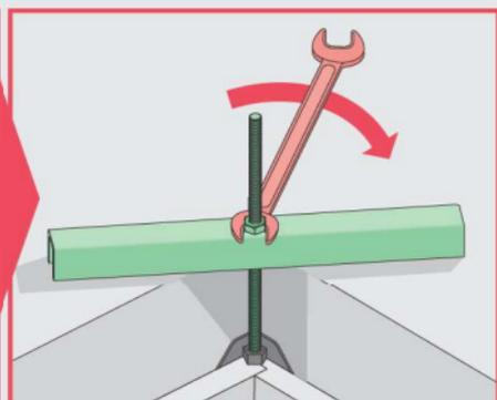
US Tighten the nut on each bracket to level the ladder on desired depth
