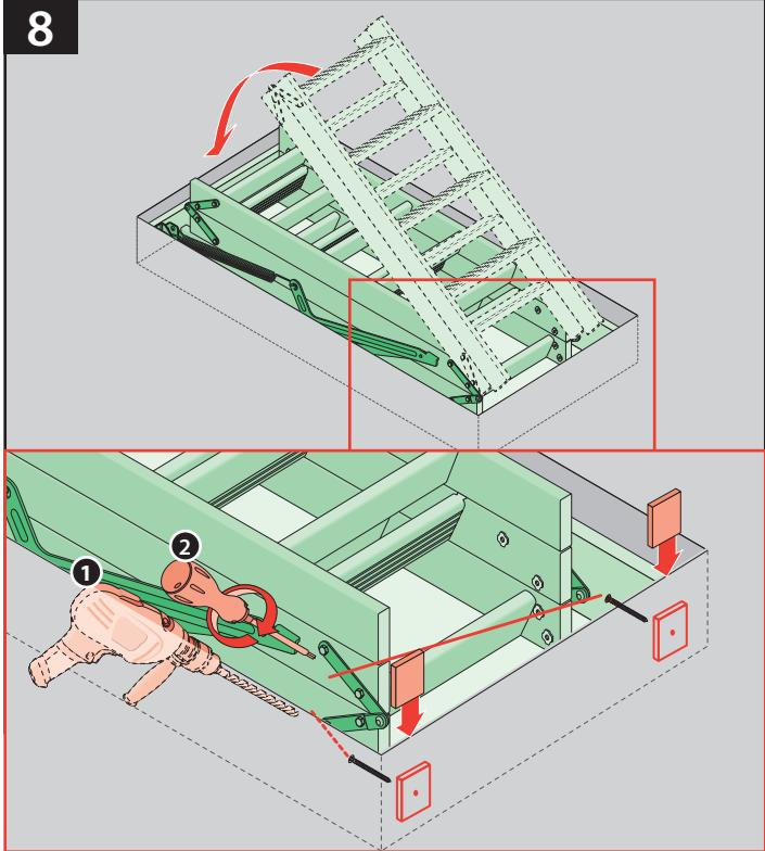
**US** Check diagonals and adjust installation screws if necessary
