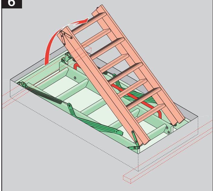
**US** Use shims with all installation screws to prevent frame bowing
