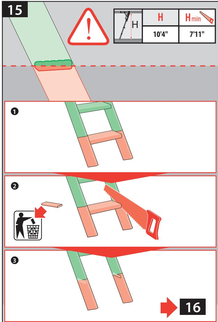
**US** Last ladder section should have minimum two steps left after cut
