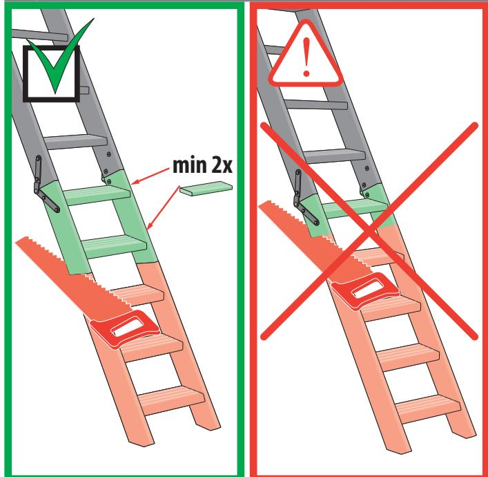
**US** Carefully unfold the ladder while bending the last section to the back as shown on step 14
