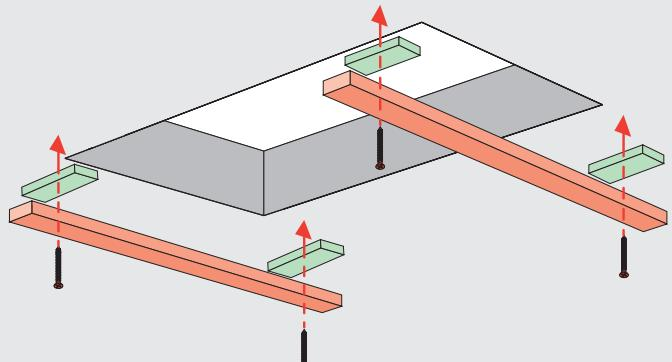
**US** Use a distance block 'T' to level ladder frame with a ceiling drywall.
