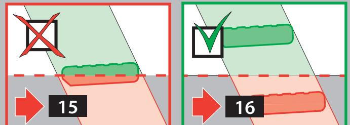
**US** In case when cut line aligns with ladder step, remove that step - as shown in section 15
