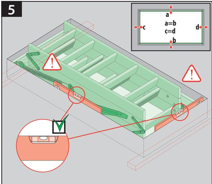
**US** Lift two ladder sections to install first installation screws
