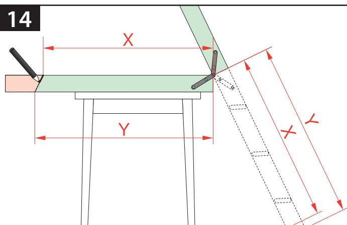
**US** Measure required distance to the finished floor. Transfer the measurements onto last ladder section as shown above.
