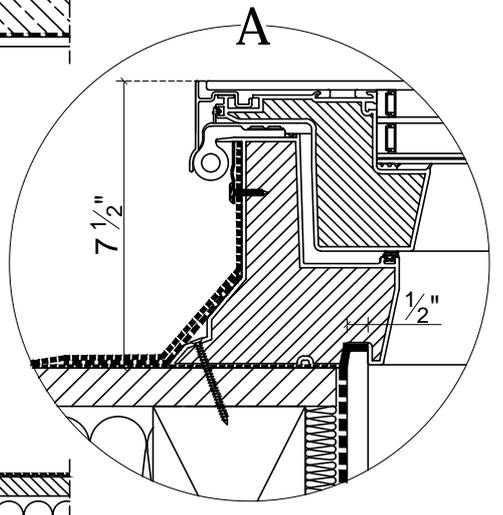
735-DRF DU6 FAKRO flat access roof light opened manually, glazing unit DU6
