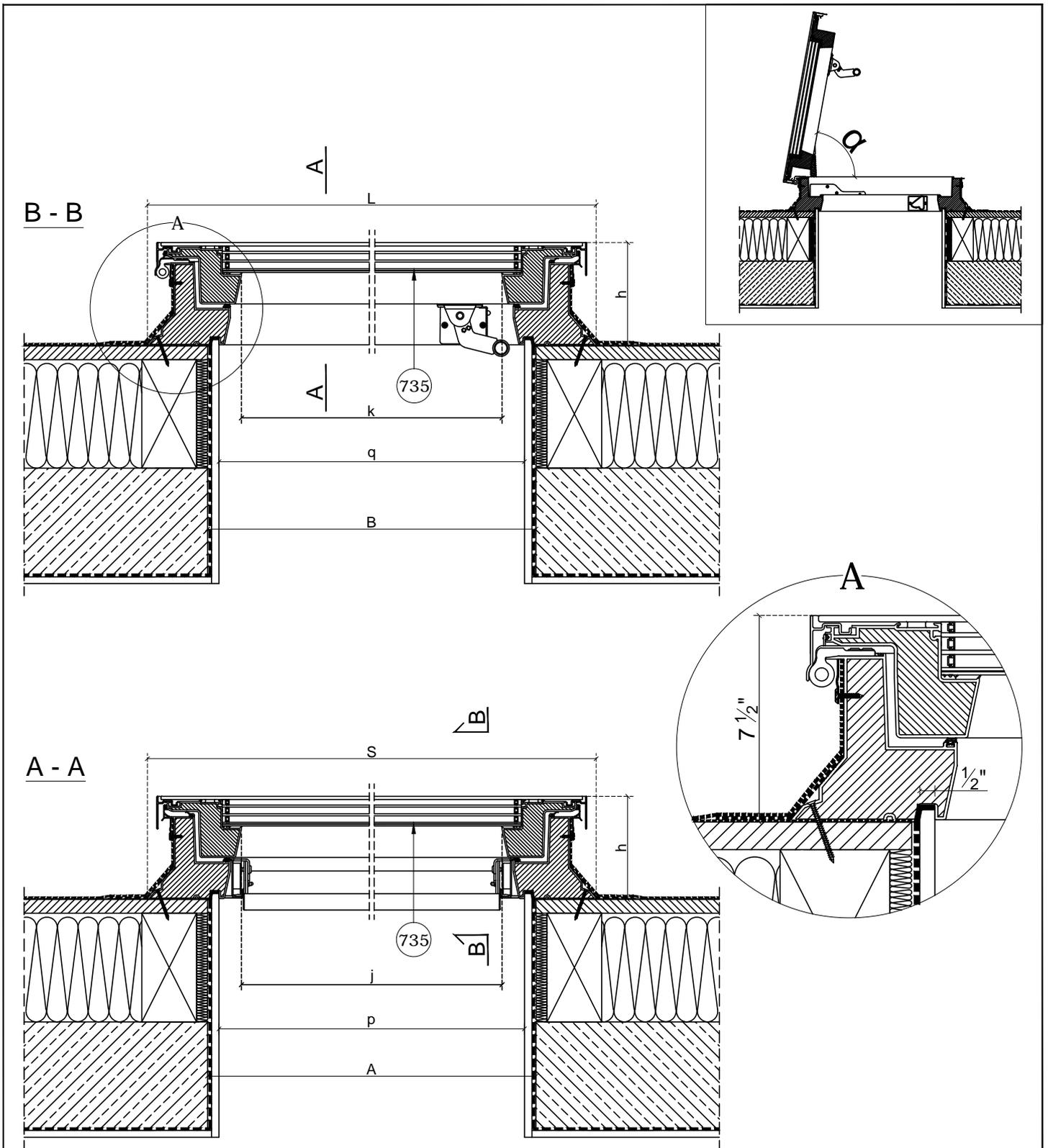
735-DRF DU8 FAKRO flat access roof light opened manually, glazing unit DU8
