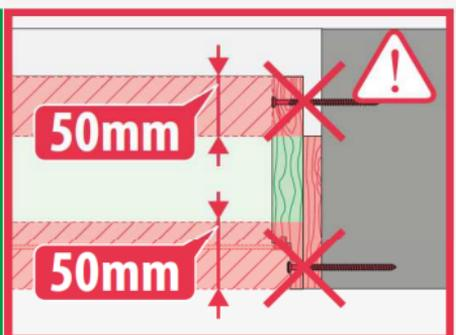
US The stairs must not be used unless they are anchored to the ceiling in accordance with the instructions shown above.
