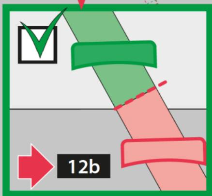
US To avoid cutting the ladder on the step, screw in the adjustment screws. Verify if both screws are properly adjusted. Note: When changing the angle of the ladder with the adjustment screw, it is forbidden to unscrew the screw further than 3/8" as shown in the figure below.
