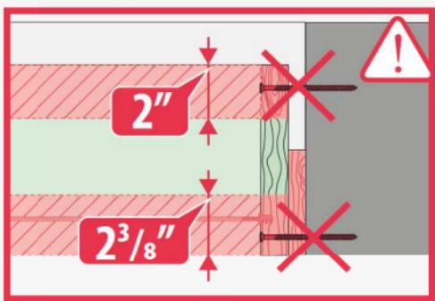
US The stairs must not be used unless they are anchored to the ceiling in accordance with the instructions shown above.
