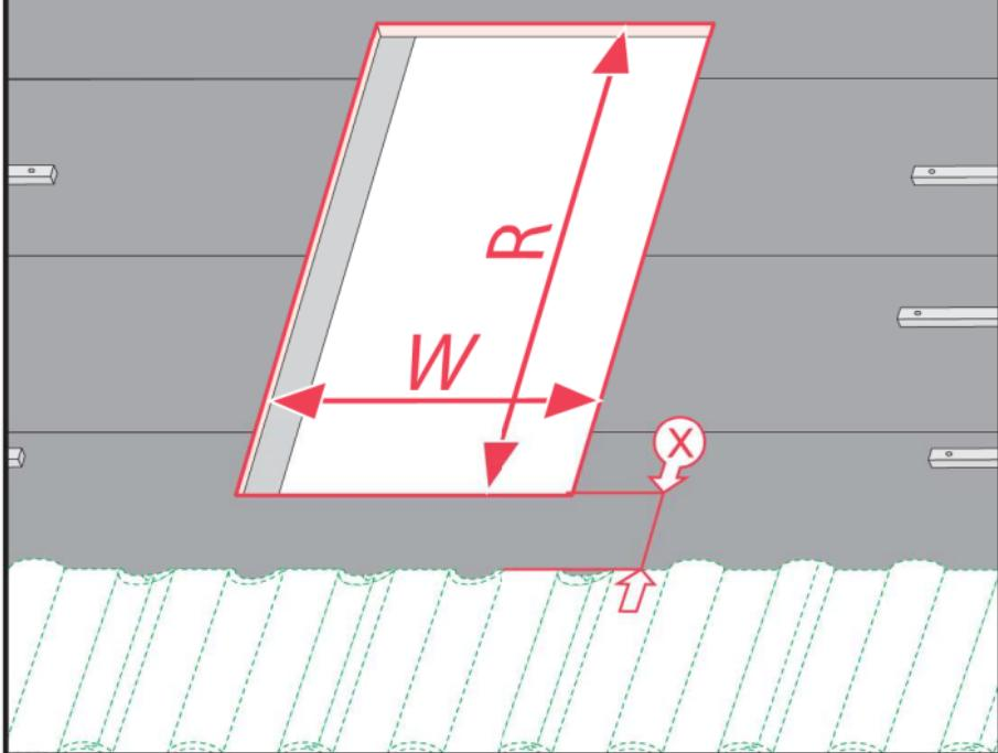
**US** Prepare the rough opening in the roof using the WxR dimensions (dimensions W and R are provided in the table on page 2). Place wooden battens around the opening. Battens should be of the same thickness as battens used for roofing material.
