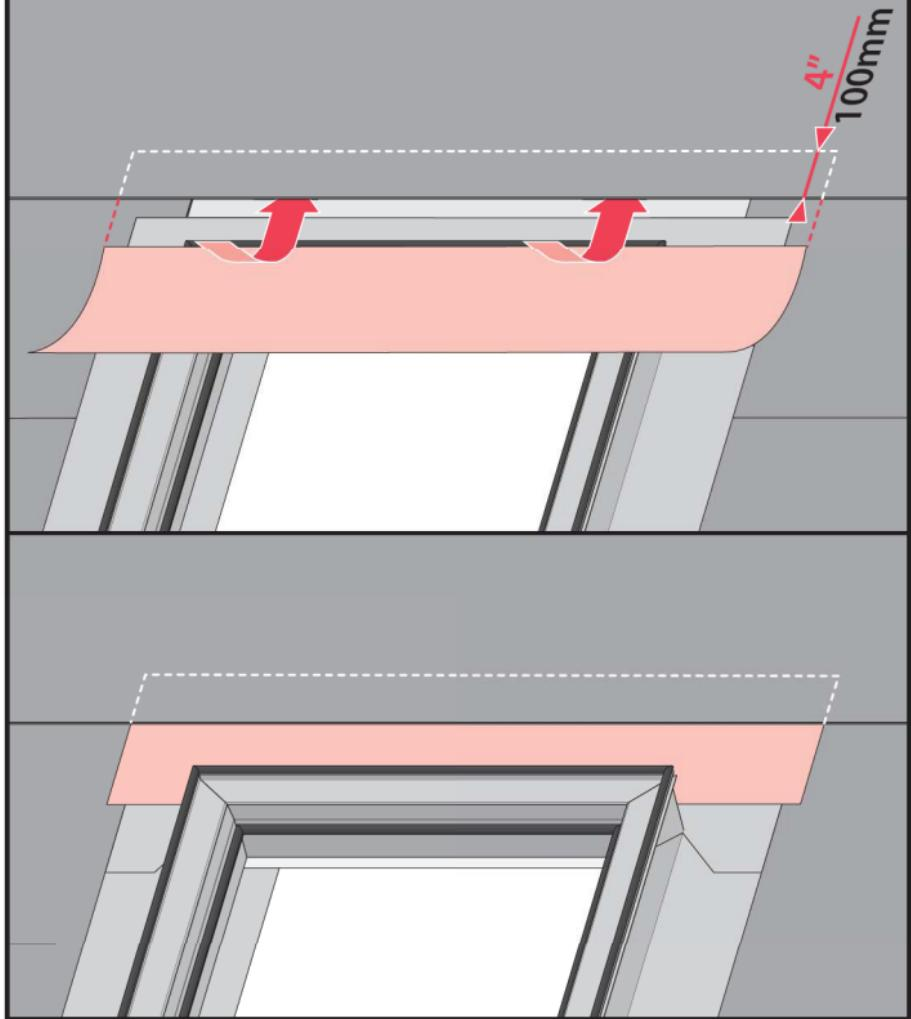
US To ensure proper water drainage, interweave the skylight's underlayment with the new roof underlayment (new construction).
