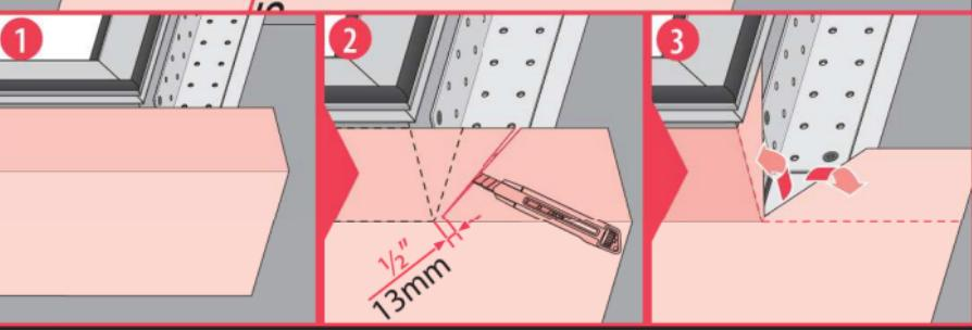
**US** For complete waterproofing, apply self-adhesive underlayment (separate purchase) starting at the bottom of the skylight.
