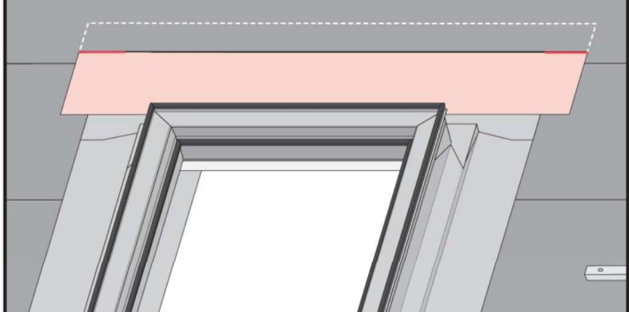
**US** To ensure proper water drainage, interweave the skylight's underlayment with the existing roof underlayment (retrofit).
