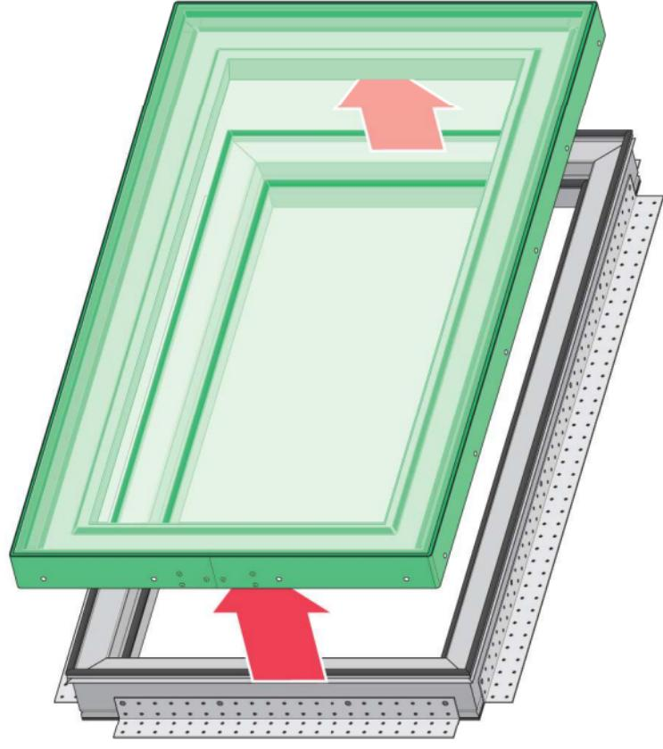
US Remove the skylight sash from the frame.
