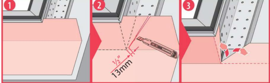
**US** For complete waterproofing, apply self-adhesive underlayment (separate purchase) starting at the bottom of the skylight.
