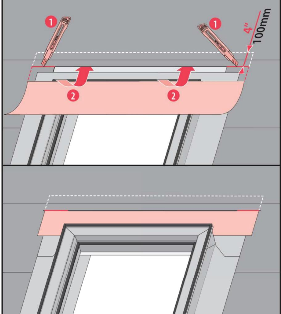
US To ensure proper water drainage, interweave the skylight's underlayment with the existing roof underlayment (retrofit).
