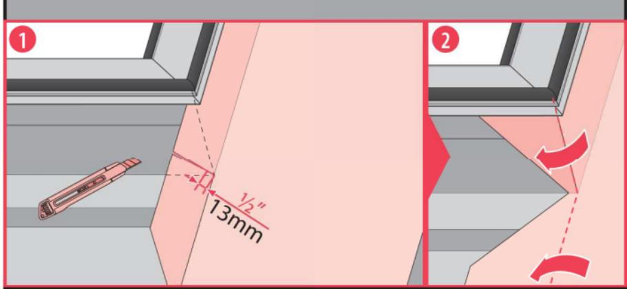
**US** Apply self-adhesive underlayment on the sides of the skylight .
