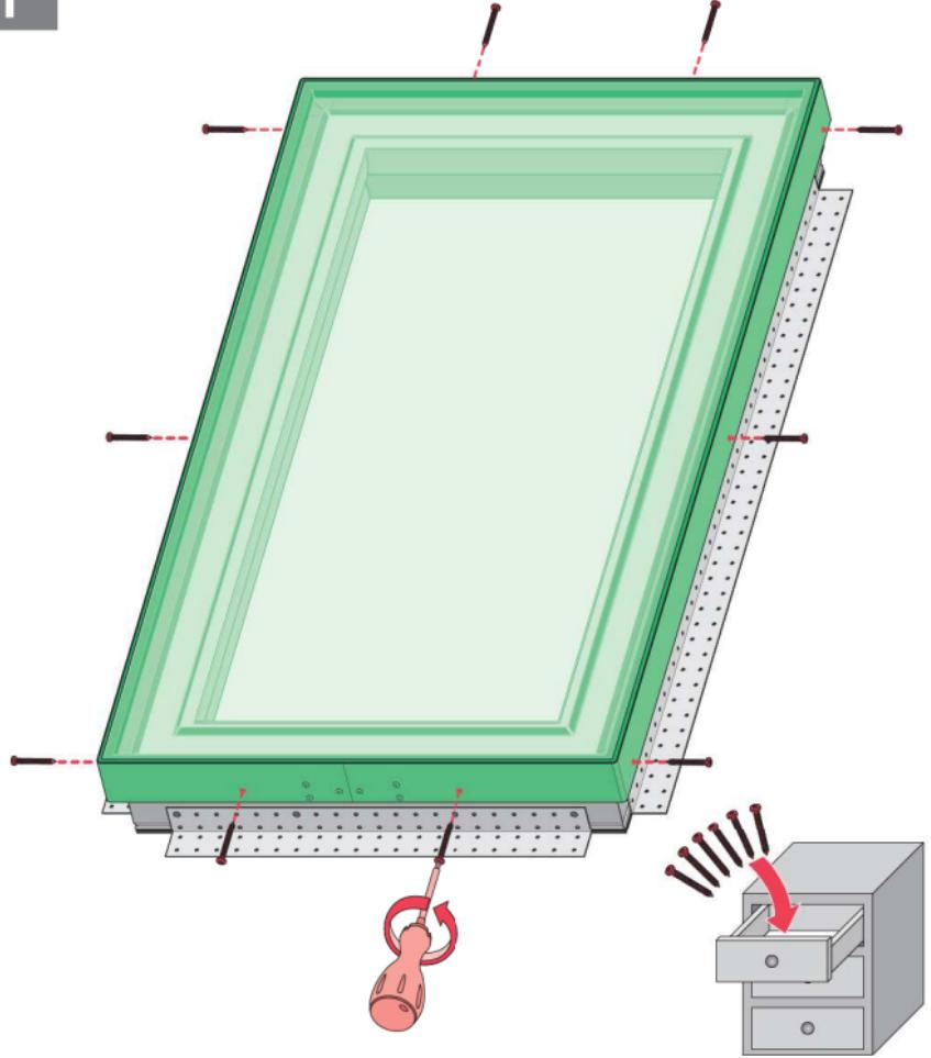
US Remove and save all the screws fastening the skylight sash.
