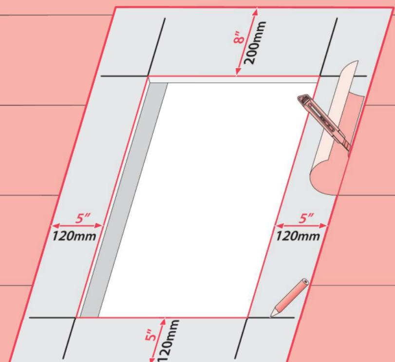
**US** Remove existing roofing underlayment around the opening.
