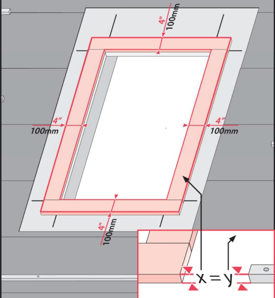
**US** Place 4" (100mm) wide battens around the rough opening. Skip this step if your roof has no battens. Battens should be of the same thickness as battens used for the roofing material.
