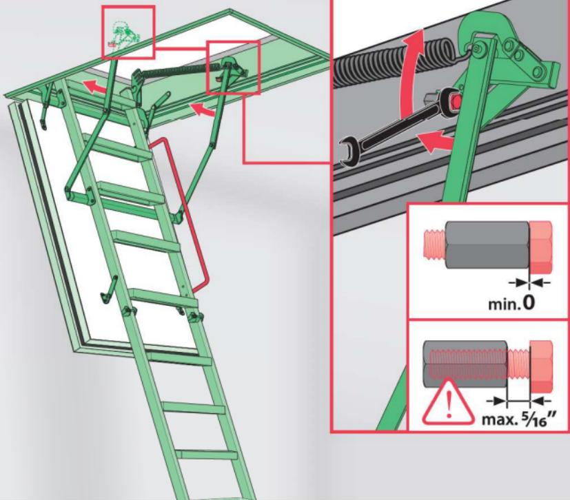
**US** To avoid cutting the ladder on the step, screw in the adjustment screws. Verify if both screws are properly adjusted. Note: When changing the angle of the ladder with the adjustment screw, it is forbidden.
