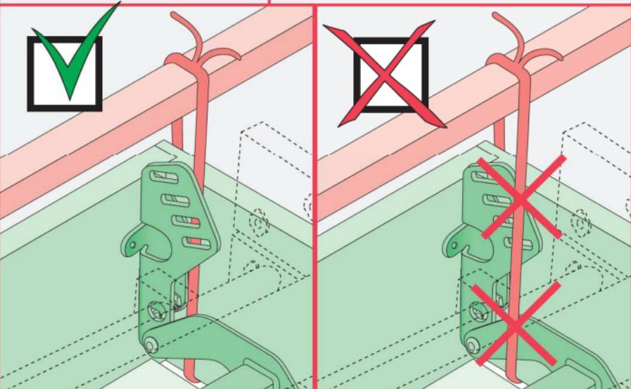
US 1) temporary installation brackets - check floor cross section requirements
