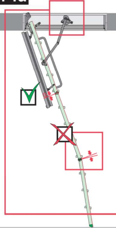
US The ladder is too short - screw in the adjustment screw.
