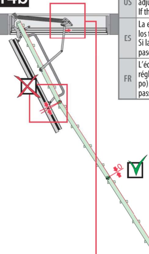
US The ladder is too long - unscrew the adjustment screws. Note: no more than 5/16". If the ladder is still too long go to step 13b.
